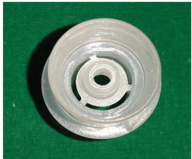
Figure 1. Photograph showing the normal connector showing patency for the inner (FGF) as well as patency for the expiratory (corrugated) tubing.
