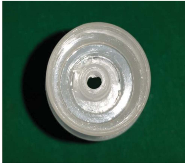
Figure 2. Photograph showing the defective connector with patency for the inner (FGF) and non patency for the outer (corrugated) tubing.
